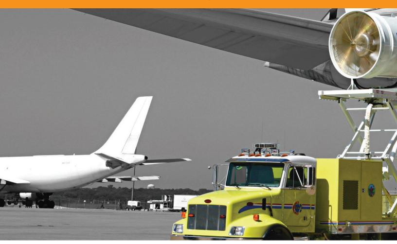
The powerhouse of our ventilation line, the *TEMPEST* MVU® 60 is the largest unit we manufacture. The combined massive 60" (1.5 meters) seven (7) blade aluminum impeller, and steel shroud are capable of generating air movement unlike any other ventilation unit. At a calculated 400,000 Open Air Flow CFM (679,000 m³/hr), the MVU®60 will ventilate nearly anything caught downwind from it.
