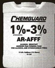
Chemguard's Ultraguard 1%-3% proportions 1 part concentrate to 99 parts water for hydrocarbon fuels and 3 parts concentrate to 97 parts water for polar fuels. This agent is intended for topside use on type II and type III applications.
