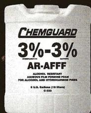
Chemguard's Non Sprinkler AR-AFFF proportions at 3 parts concentrate to 97 parts water for hydrocarbon and polar fuels. Specifically formulated for topside use on type II and type III applications.
